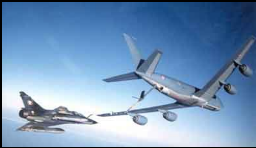
A MIRAGE 2000 N of the EC 2/4 "La Fayette", flying back from "Red flag" manoeuvres in the US. The aircraft is refueled by a French Strategic Air Forces C-135FR Stratotanker
